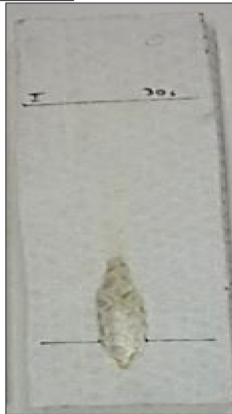
Flame during 30s / Flamme appliquée pendant 30s
